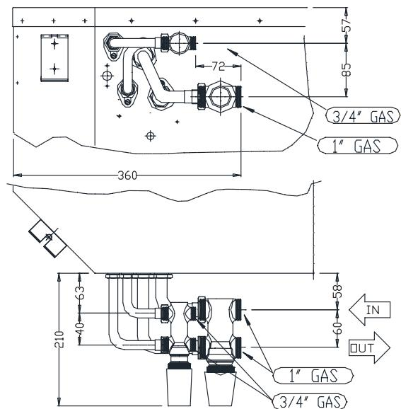
**DIVA 60÷110 avec vannes 2 voies ON/OFF****DIVA-I 60÷110 avec vannes 2 voies ON/OFF****Installations à 2 tuyaux**
